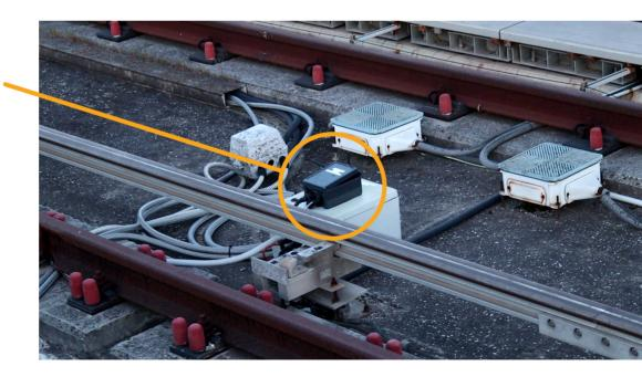
A simulated signalling asset with a wireless communication device used to test connectivity with a drone hovering over it.
